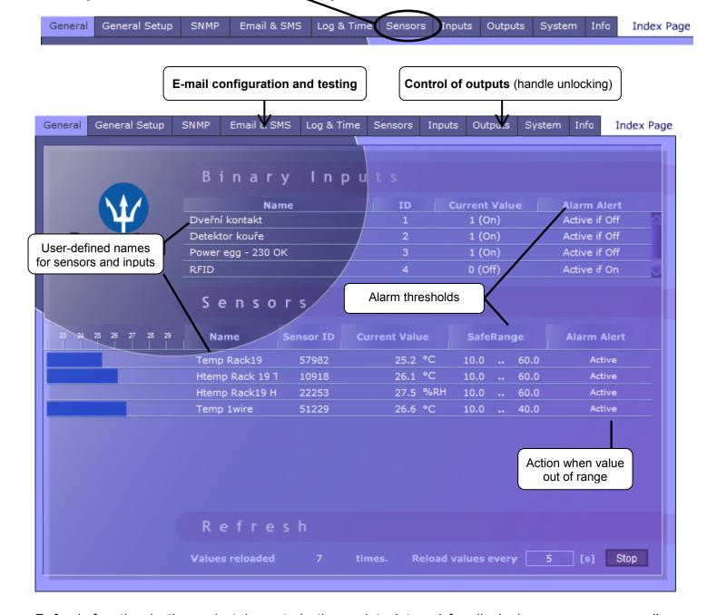
Refresh function in the main tab controls the update interval for displaying new sensor readings.
