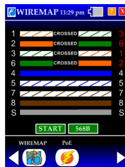
Example - Crossed 12-36 shielded cable
