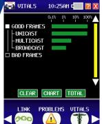
Vitals provides an indication of the operational condition of a network. A real time analysis of good and bad frames received is used to determine if the network is healthy or problems exist that may be affecting performance.
